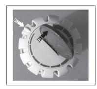
**Example:** To set a decrease in temperature of –3K, start at the preset point and turn the device clockwise up to the third blue marking interval.
